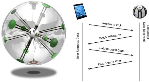
**Figure 1: (a) Adidas micoach smartball; (b) The (inferred) protocol between the app and the ball to initiate a kick and gather the corresponding accelerometer readings.**
