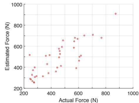
**Figure 2: Actual vs estimated force when the soccer ball is dropped on the force-pad from various heights.**
